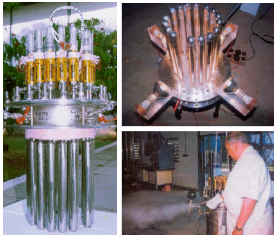
Figure 2. Evacuated and sterilized cryoprobes. (Left) Assembled in a manifold ready for immersion in liquid Ne for launch. (Top right) Heat sterilization under vacuum in an infrared set-up at 140°C. (Bottom right) Steam sterilization procedure.
