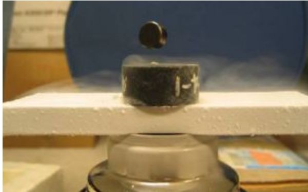
Magnetic levitation in a high temperature superconductor.
